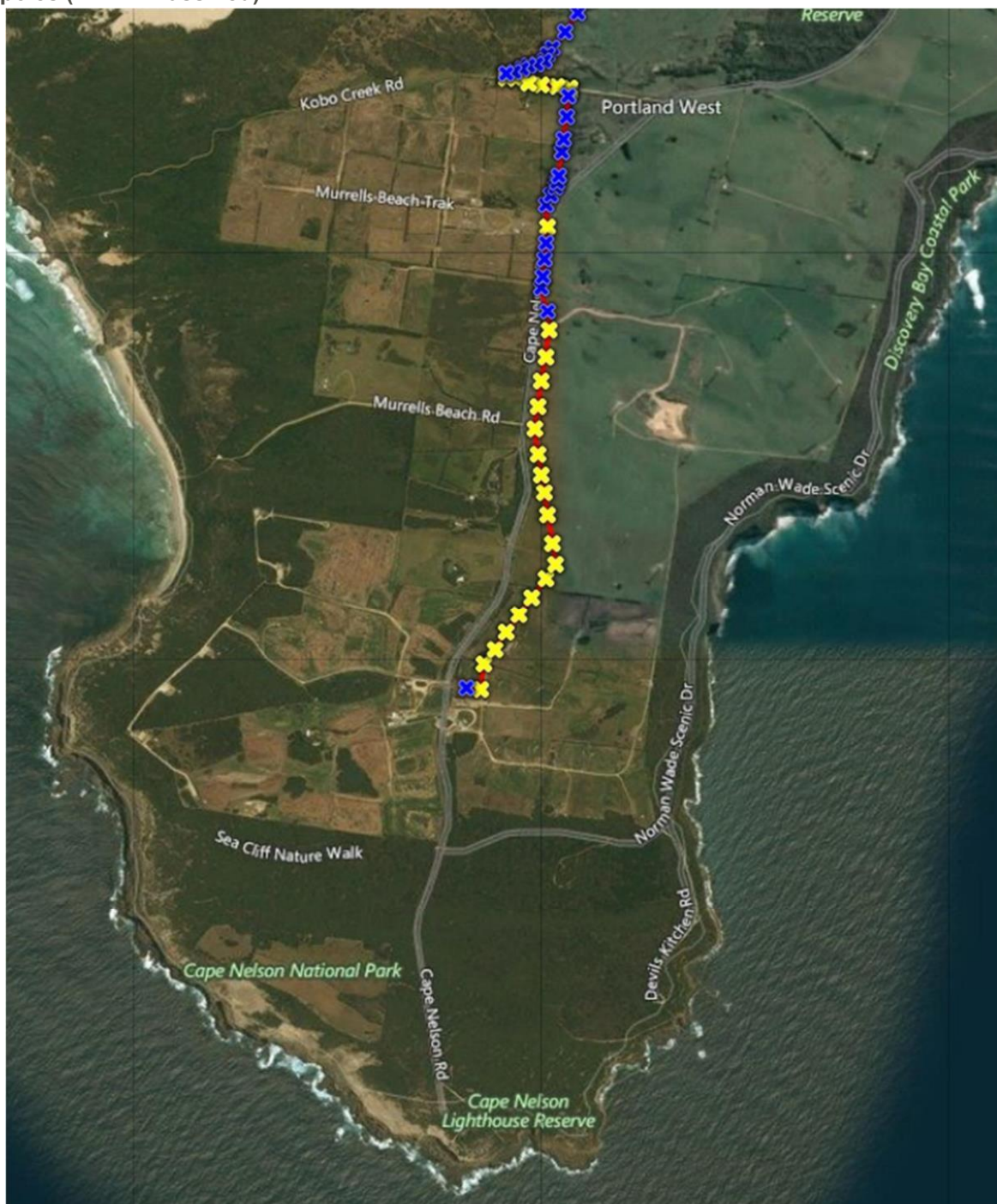
Appendix A.3 Cape Nelson South Site Layout showing the location of the electric lines and poles (HBRA Classified)
