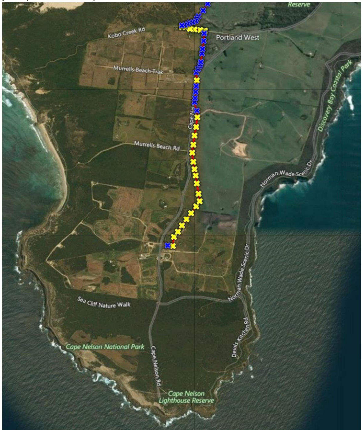
Appendix A.3. Cape Nelson South Site Layout showing the location of the electric lines and poles (HBRA Classified)
